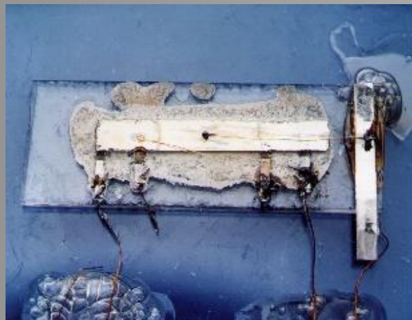
The first integrated circuit (Texas Instruments, 1958)
