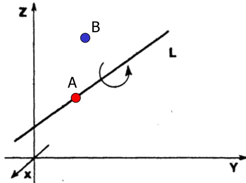
$$[R_x] = \begin{bmatrix} 1 & 0 & 0 & 0 \\ 0 & \frac{n}{d} & \frac{m}{d} & 0 \\ 0 & -\frac{m}{d} & \frac{n}{d} & 0 \\ 0 & 0 & 0 & 1 \end{bmatrix}$$
